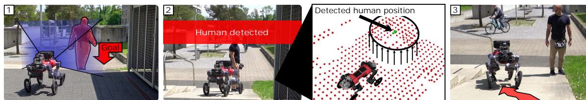
Figure 4: Obstacle negotiation. (A) Navigating around blocked routes by actively exploring the area and finding alternative paths. (B) Safely traversing a narrow space. (C) Our robot exhibits two different ways to traverse the complex obstacle. (C, D) Our robot shows an asymmetric understanding of traversability, being able to traverse higher steps when going down. (E) Ensuring safety around humans by incorporating additional human detection and overriding height scan values.
